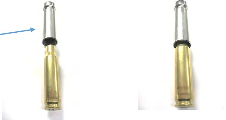
Rifle case neck fits up inside Caliber Specific Powder Funnel to Activate Powder Measure
