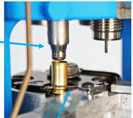
Case entering Powder Die at Station 2 on down stroke
