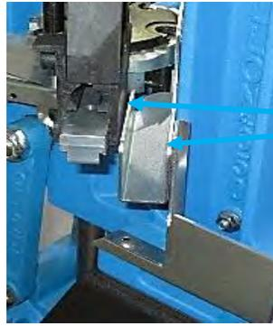
Chute/Bin Bracket not touching the Casefeed Slide when installed
