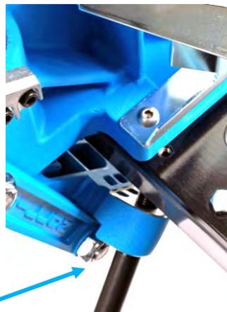
**Note  $\frac{3}{4}$ " clearance required for the Crank and Operating Handle if mounting XL750 base directly to the bench**
