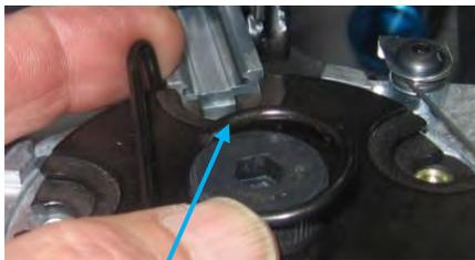
Remove Ejector Wire
