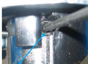
Loosen Set Screw with an Allen wrench
