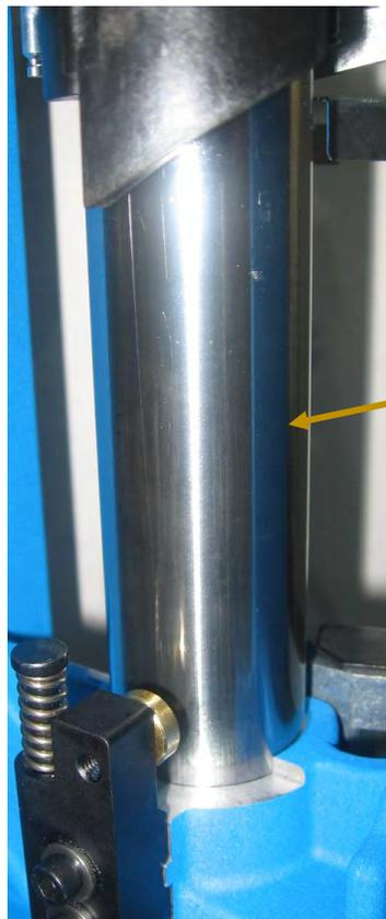
Use only 30 weight motor oil. DO NOT use a penetrating lubricant such as WD-40, Breakfree, etc.
