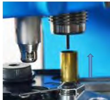
Station 1-Case Inserted into Size
