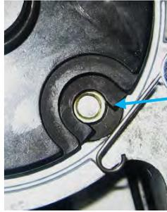
Primer Cup fits Hole in Platform without dragging and is concentric with the "U" shaped Shellplate opening/slot
