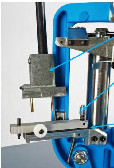
Remove all together--Primer Mag Shield, Cap, and Early Warning Alarm Assembly.
