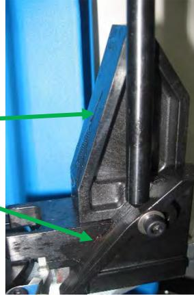
**12.2 Lightly Oil Mainshaft every 5000 Cycles--Keep clean by blowing off with compressed air frequently**
