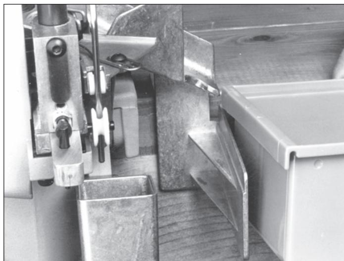
**Fig. 3 – The cartridge collection bin (#13839) simply slides onto the bracket and will be in the proper position.**
