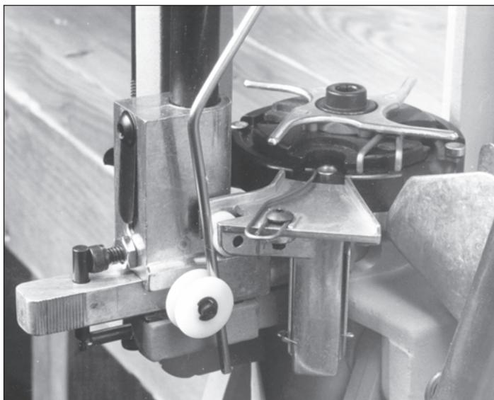
**Fig. 11** – This is the proper alignment of the operating rod and the position of the primer slide fully forward with the primer seating cup in the lowered platform.
