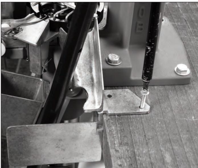
**Fig. 2 – This photograph shows the correct mounting position of the cartridge collection bin bracket in relation to the machine.**
