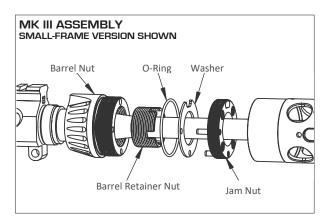
3. Clean the threads on the receiver barrel collar with a brush and solvent. We also recommend removing any Teflon® coating on these threads with a steel brush to help the thread locker bond. Coat these threads with Loctite® 271 and then install the Barrel Nut by turning it down until it stops and then backing it off until the gas tube holes are in alignment.
